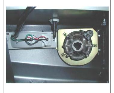
9. Placing the original bumper bar face down on a blanket remove all of the screws that hold the painted outer section to the main bumper. Using pliers remove the clip that holds the washer nozzle in the bumper and take out the nozzle (both sides). These are re-fitted into the bar once the fog lamp and turn signal are installed.
