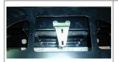
20. Fit control box bracket to bar using 8mm hardware.
